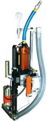
Custom Drill and Countersink solution that took a 3 step process down to one step with vacuum, error proofing and enhanced ergonomics
