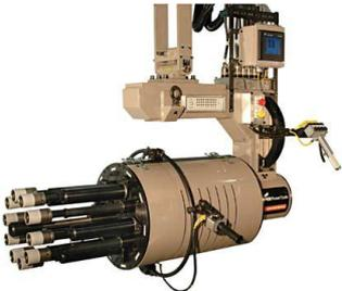
Custom 10 Spindle wheel multiple solution with advanced tightening strategies, error proofing and data collection for optimum quality
