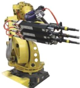
Multi Spindle Robot end effector solution with advanced tightening strategies, error proofing and data collection, reconfigurable for optimum productivity
